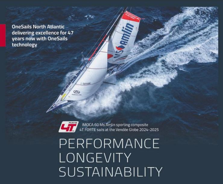
These core characteristics of 4T FORTE have been successfully tested in oceans all over the world. Unlike more traditional sail-making methods, 4T FORTE is made from high modulus fibres in a composite structure. A core, continuous yarn structural grid takes care of the principal loads, whilst micro layers provide strength in secondary directions.
